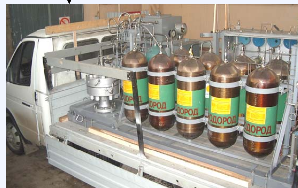
Hydrogen delivery in cylinders
