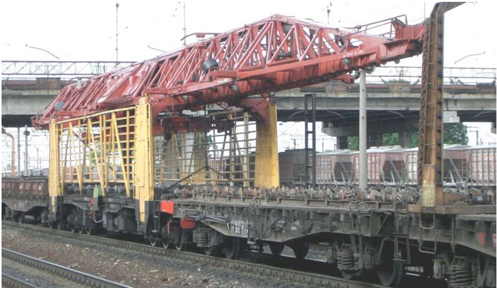
track-laying crane UK-25, converted for electric operation
