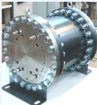
Hydrogen generation onboard (using electrolyzer)
